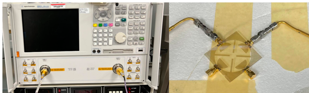
Figure 5. S-parameters measurement setup.
