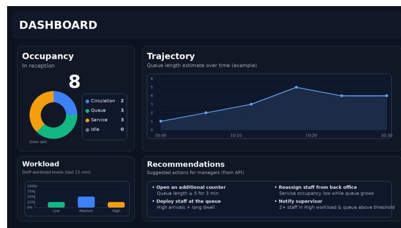
Figure 4. Prototype dashboard view rendered by the front-end consuming the DT API: OCC-derived zone occupancy, DT-inferred queue dynamics, wearable-based workload distribution, and rule-based manager recommendations over fused state.
