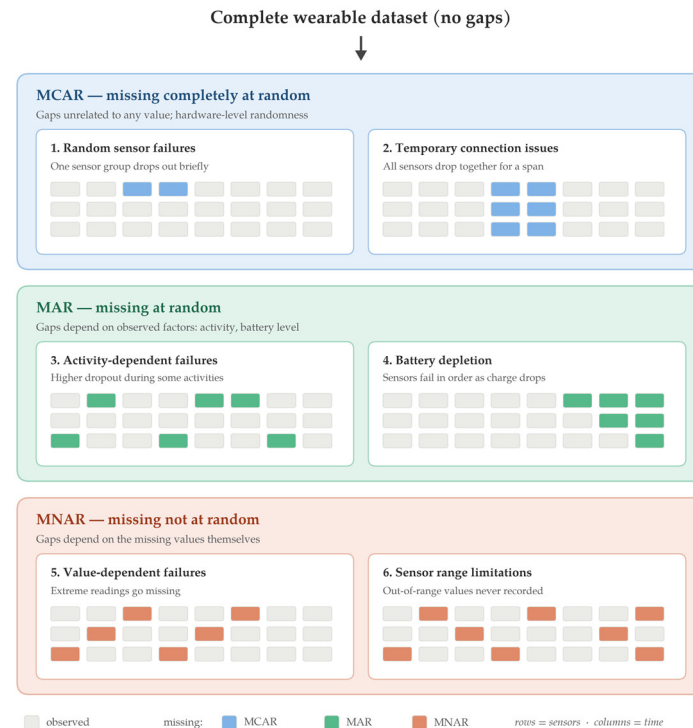
Figure 1. Overview of the six realistic missing-data scenarios, grouped by the three mechanisms of Rubin’s taxonomy (MCAR, MAR, MNAR). In each grid, rows correspond to sensor groups and columns to time; grey cells denote observed values and coloured cells denote missing values, illustrating the characteristic gap pattern of each scenario.
