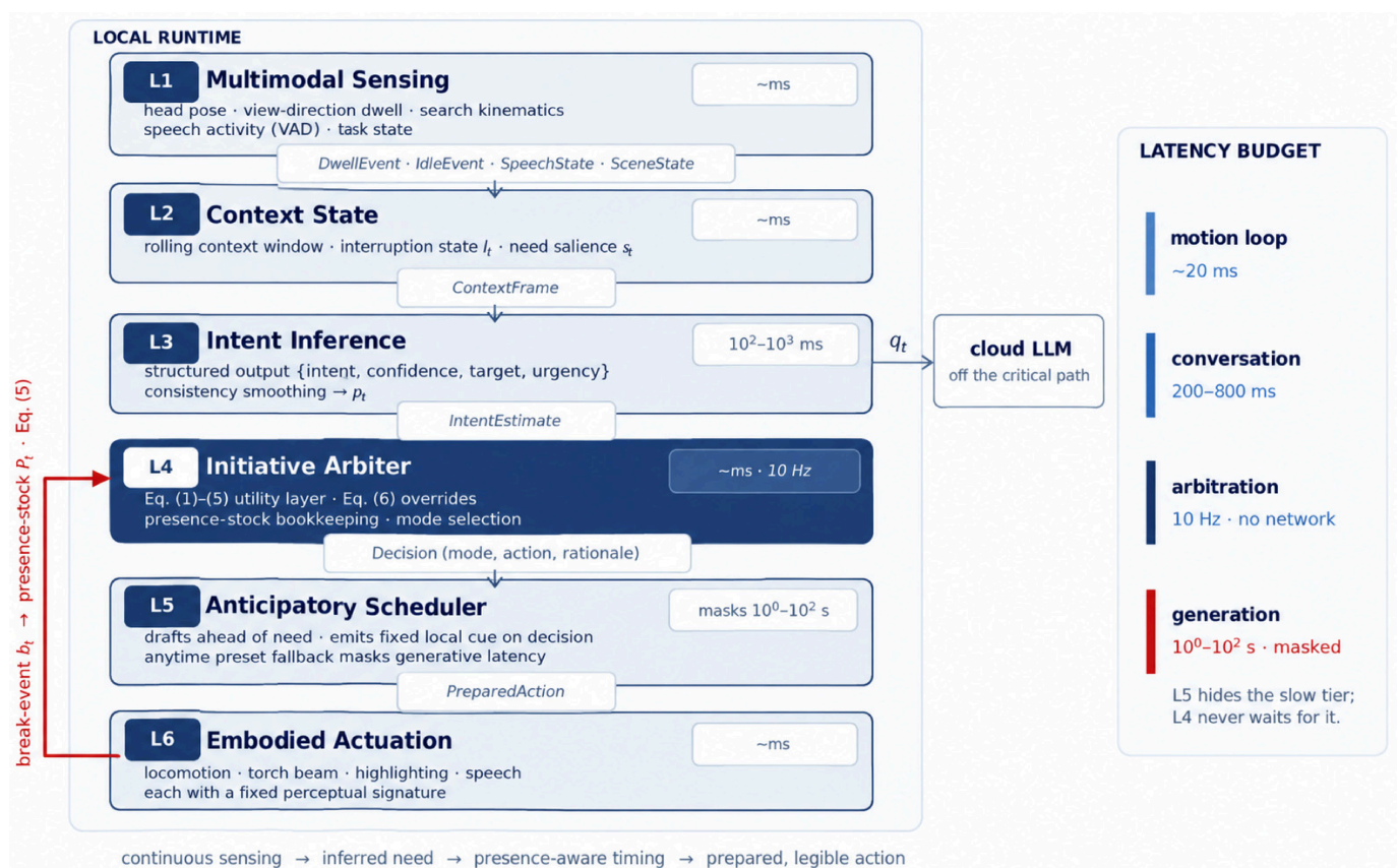
Figure 2. Agentic Presence’s reference architecture. Six typed layers connect sensing to embodied actuation. L4 evaluates the initiative policy at 10 Hz without a network call; L5 schedules prepared output. The feedback path updates the internal presence-risk stock after an intervention issued at high estimated interruption.
