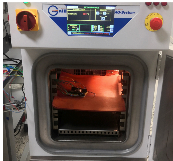
Figure 11. Thermal chamber and instrumentation used for the measurements from -40 °C to 150 °C.
