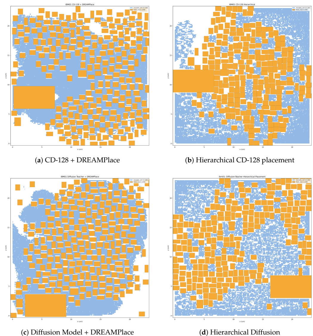
Figure 3. Full-circuit placement visualizations for IBM01 under four learned placement flows. (a) CD-128 generates the macro placement before DREAMPlace performs standard-cell placement. (b) Hierarchical CD-128 places macros and clusters globally, followed by cluster-local standard-cell optimization and full-chip assembly. (c) The diffusion model generates the macro placement before DREAMPlace performs standard-cell placement. (d) Hierarchical diffusion first places macros and clusters globally and then performs cluster expansion, local optimization, and final assembly.
