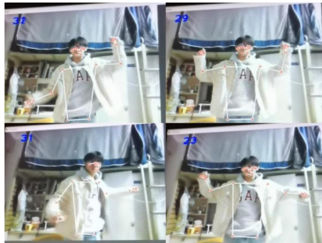
Figure 7. Human key-point recognition effect of front camera images.
