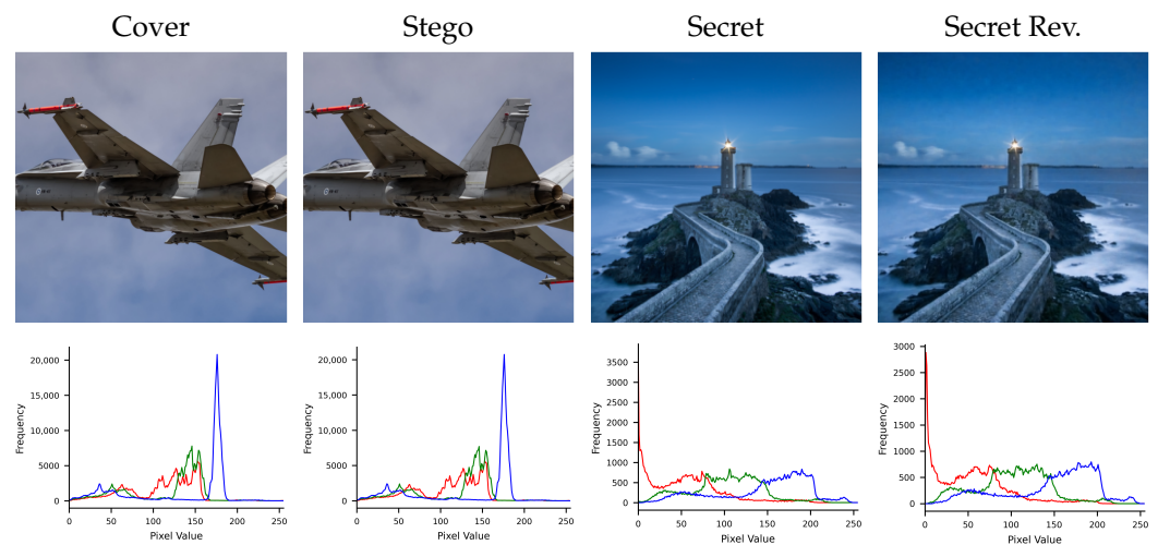
Figure 5. Comparison of RGB-channel histograms for representative experimental images. The first row shows the original images, and the second row shows the corresponding RGB-channel histograms (red, green, and blue curves represent the respective color channels).
