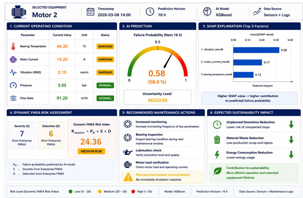
Figure 3. Example of a predictive maintenance dashboard based on real operating data.
