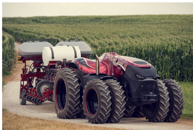
Figure 11. Automated tractors equipped with GPS and B-IoT for real-time data collection and field mapping [160].
