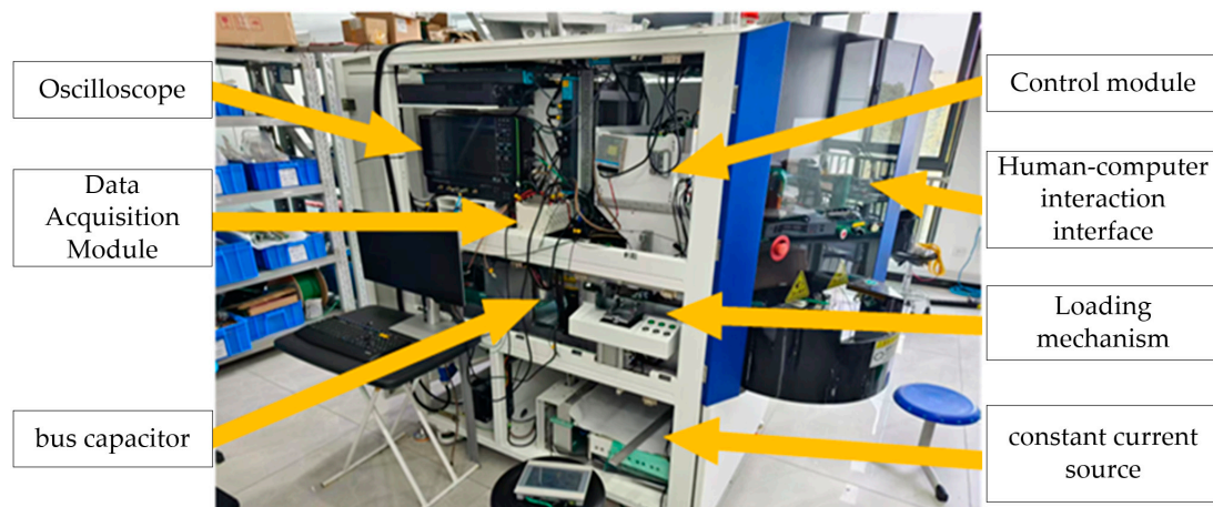
Figure 3. Physical prototype of the dynamic-static test machine.
