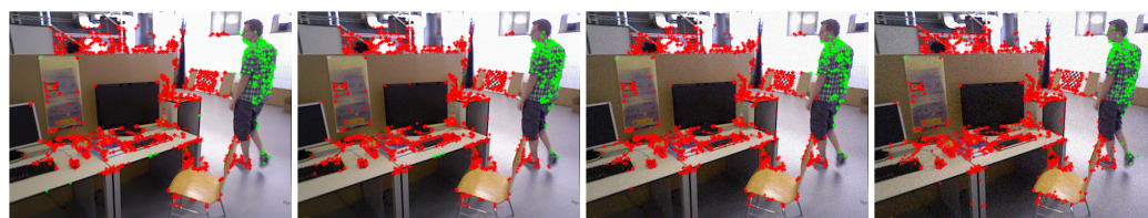
Figure 8. Effect of Gaussian noise on dynamic feature point detection. Static and dynamic feature points are shown in red and green, respectively. The same image frame is used in all cases to isolate the effect of noise.
