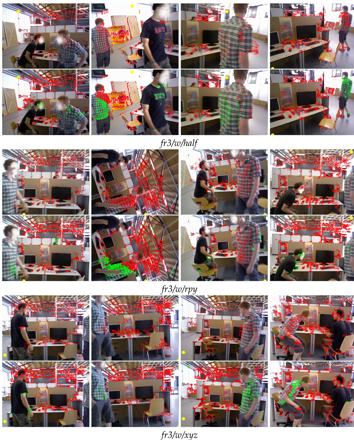
Figure 6. Optical flow vectors of feature points, K point representing MDP, and static/dynamic labeled feature points.
