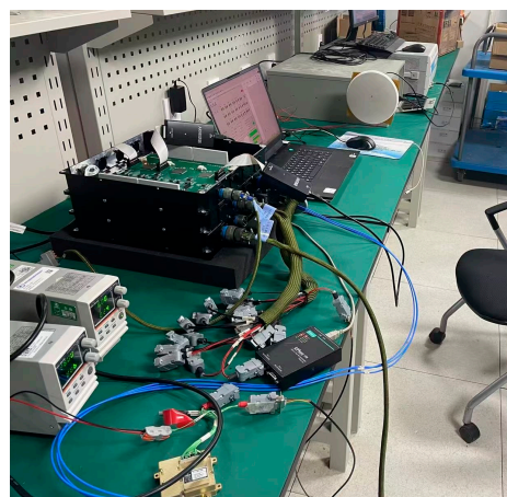
Figure 15. Hardware-in-loop test architecture with GNSS signal injection.
