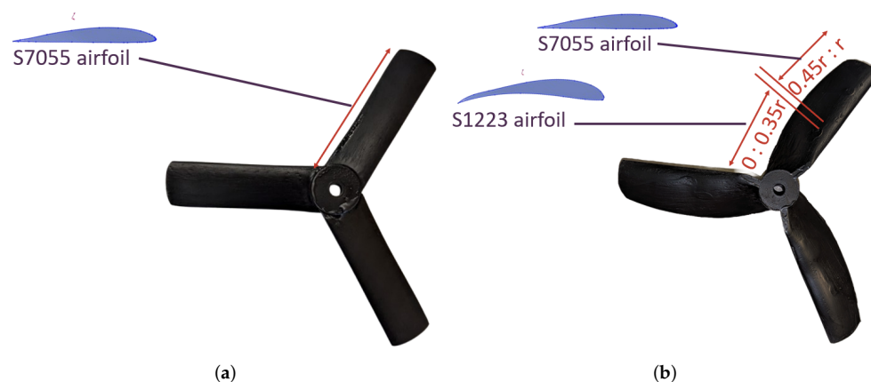
Figure 6. Selected rotors for the present study. (a) Rotor A. (b) Rotor B.
