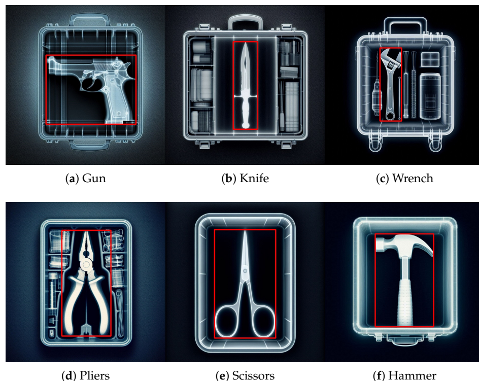
Figure 3. Examples of Gen AI X-ray images for prohibited items that we created, where the red boxes indicate the prohibited items that have been labeled.
