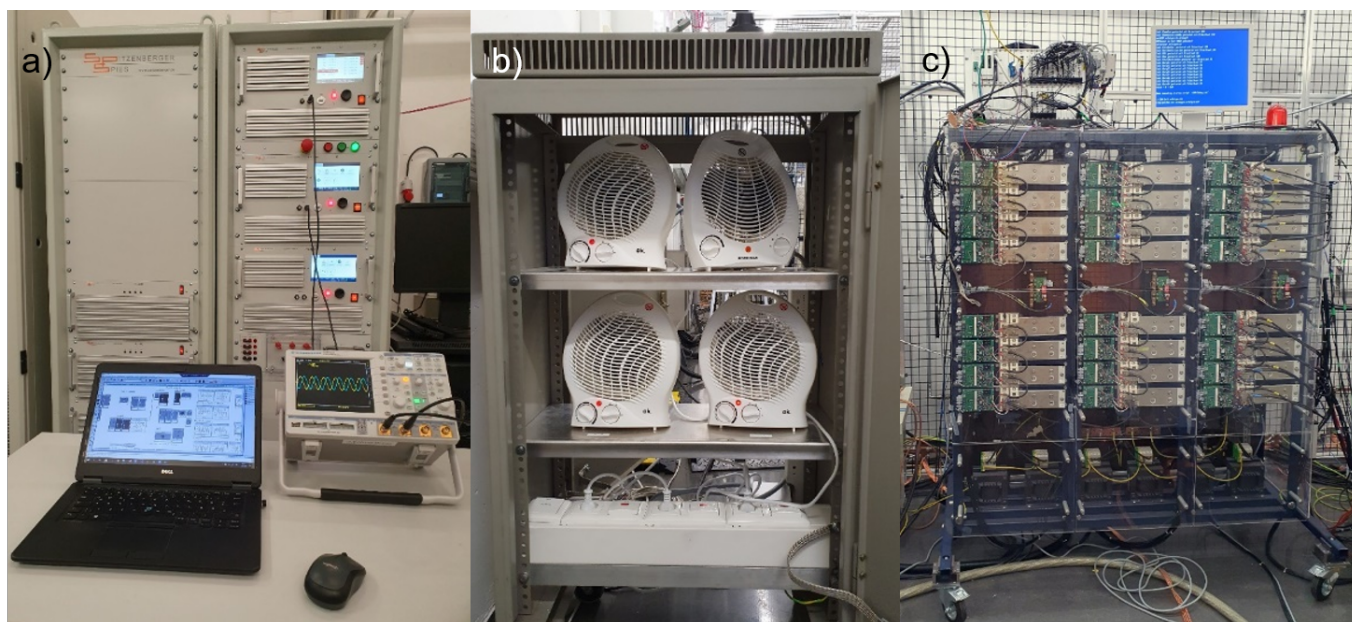
Figure 6. Connected hardware during PHIL-coupling: (a) power amplifier, (b) three-phase resistive load, (c) LabMMC connected to the Li-ion storage.
