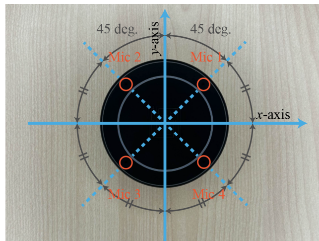
Figure 2. Microphone array with 4 elements (Seed Studio ReSpeaker USB Mic Array v2.0 [20]).
