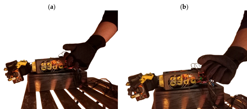
Figure 10. (a) Grasping with haptic feedback; (b) Grasping without haptic feedback.
