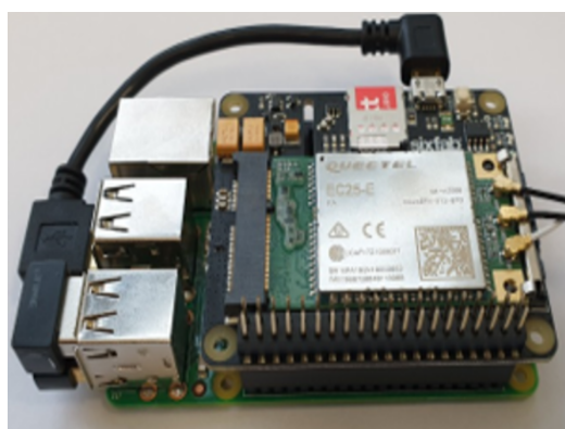
(a) Photograph of the custom signal meter.
