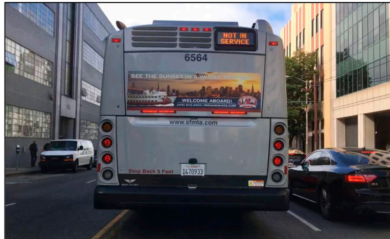
Figure 11. Failure case under severe occlusion. The bus in the foreground blocks most of the target vehicle, causing YOLOv8n to miss the detection and preventing the collision-warning system from generating an alert.
