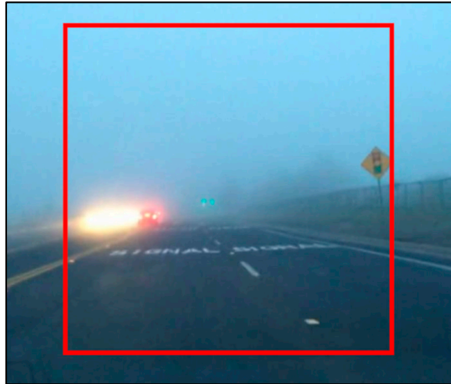
Figure 8. Detection and depth estimation failure under dense fog conditions. The low contrast and strong light scattering from fog significantly degrade visual clarity, causing YOLOv8n to miss distant vehicles and SGBM to generate unstable disparity estimations.
