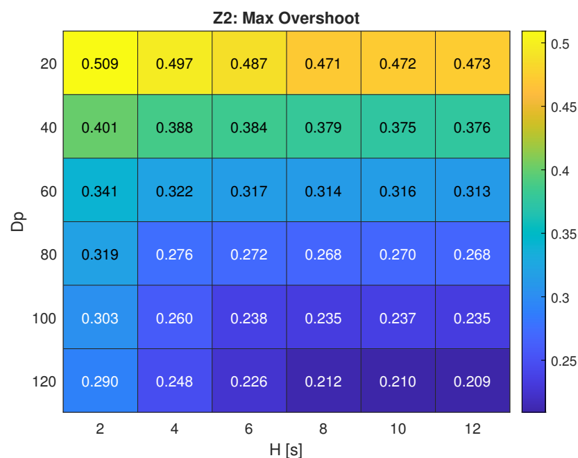
Figure 19. Maximum frequency overshoot in Zone 2 across the (H, D_p) grid.
