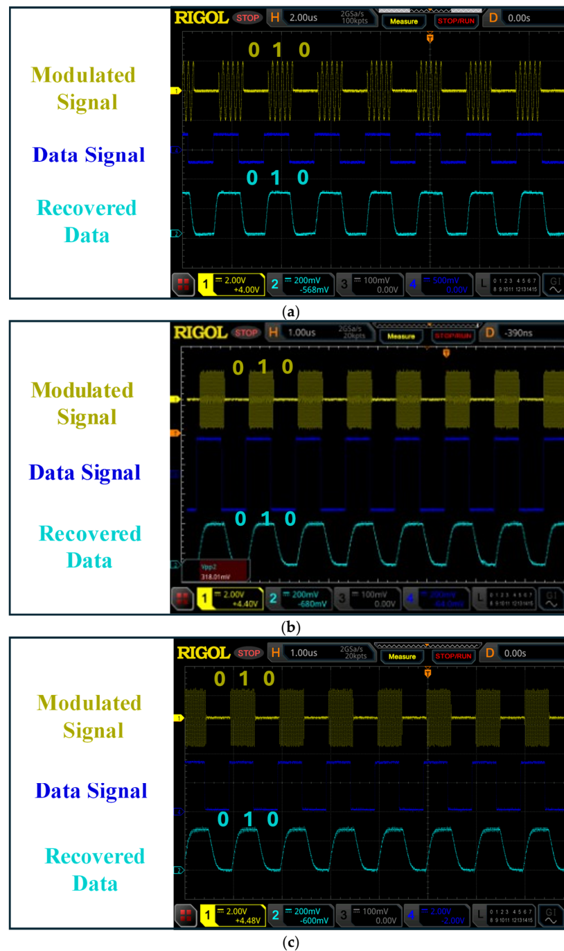
Figure 12. Measured waveforms at a 2 Mb/s data rate, displaying the ASK-OOK modulated and data signals, and recovered data for modulated signals at (a) 5 MHz, (b) 50 MHz, and (c) 150 MHz.
