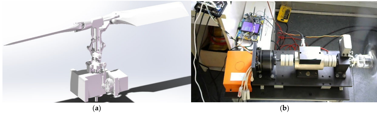
Figure 6. (a) Three-dimensional assembly of the variable pitch propeller. (b) Variable pitch propeller 1:1 test bench.
