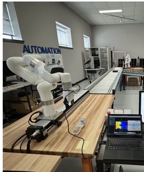
Figure 2. Experimental apparatus showing robotic arm, depth camera, control system, and object placement area.
