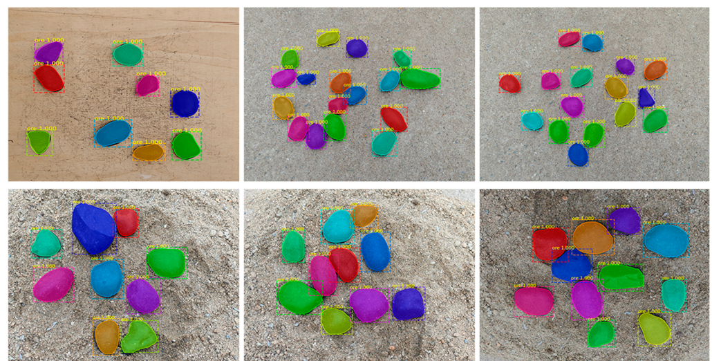
Figure 6. Segmentation results of ore detection in real-world scenes.
