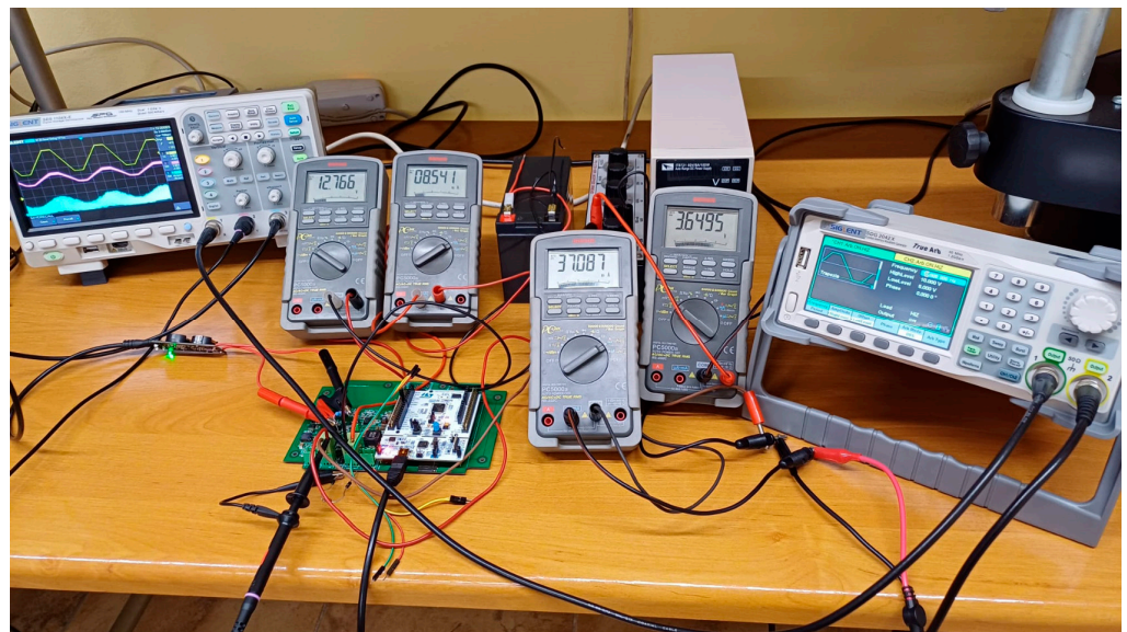
Figure 26. The prototype of the energy harvesting device during quasi-realistic tests. On oscilloscope display: yellow waveform—open-circuit voltage V_S from duplicated second channel of the AWG, magenta trace—input voltage V_C , cyan trace—inductor L current measured on a 0.1 \Omega resistor using differential probe. Meters from left: V_B [V], I_{out} [mA], I_{IN} [mA], V_{CAV} [V]. Source parameters: open-circuit voltage V_S varied from 5 V to 10 V, R_S = 100 \Omega .
