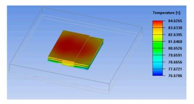
Figure 15. Optimal temperature distribution of six-layer stagger-stacked DDR module.
