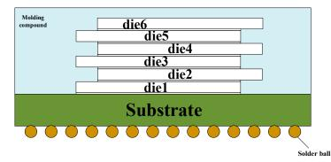
Figure 11. Schematic diagram of a six-layer stagger-stacked DDR module.
