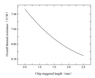
Figure 7. Overall thermal resistance vs. chip staggered length.
