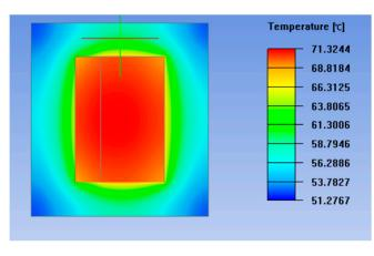
Figure 9. The optimal temperature distribution of the module.
