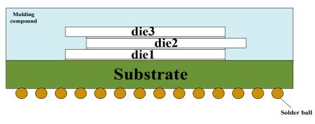
Figure 18. Schematic diagram of a three-layer stagger-stacked DDR module.
