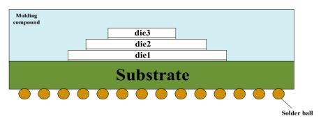
Figure 16. Schematic diagram of a three-layer pyramid package.
