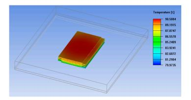
Figure 13. Initial temperature distribution of six-layer stagger-stacked DDR module.
