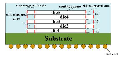
Figure 1. The whole structure of the stagger-stacked DDR module.
