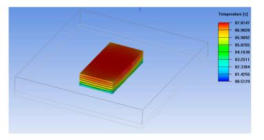
Figure 14. Optimal temperature distribution of six-layer cantilever package.
