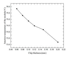
Figure 4. Junction temperature vs. chip thickness.
