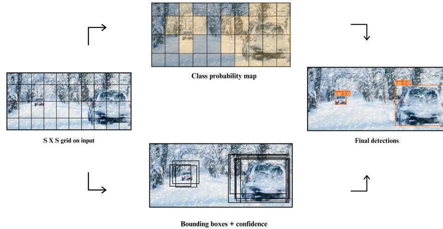
**Figure 3.** The procedure outlines the workflow of YOLOv5. Each image is segmented into uniformly sized boxes, and bounding boxes are drawn. The width of each line within the box corresponds to the confidence ratings.
