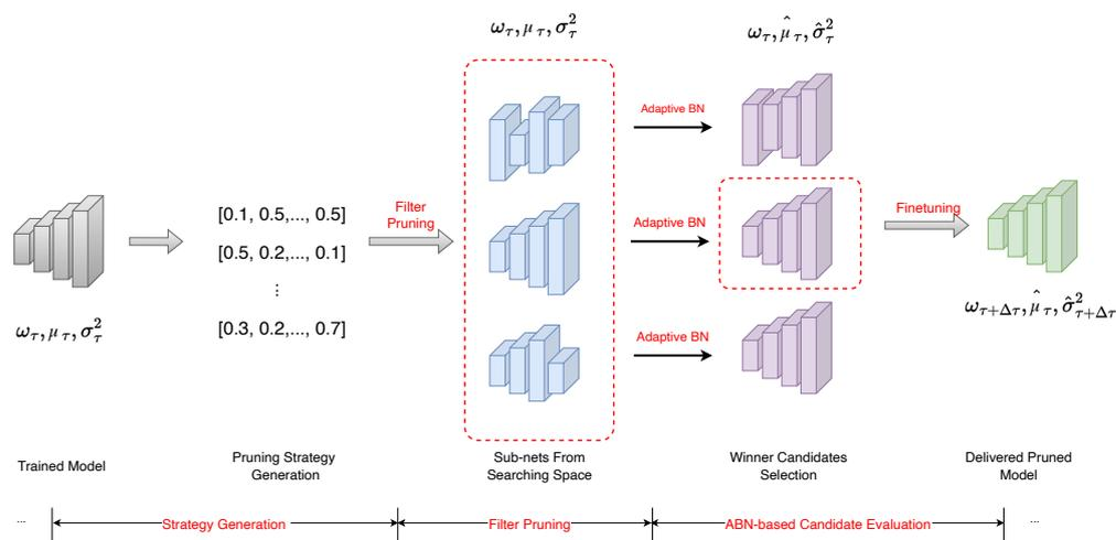
Figure 10. The pipeline of EagleEye Pruner.
