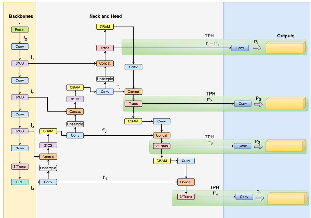
Figure 6. The architecture of the improved YOLOv5 is showcased with blue highlights indicating the integrated blocks.
