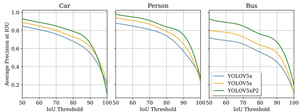
**Figure 17.** Average precision of improved models at different IoU thresholds (%).
