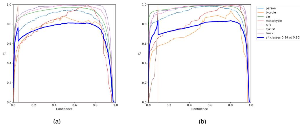
**Figure 12.** F1 curves for training our proposed YOLOv5 in small- and large-sized target, where the performance of the suggested model saturates gradually towards larger thresholds, indicating a more robust representation as (a) and (b) show.
