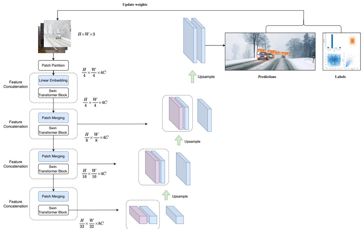
**Figure 8.** The diagram of the Swin Transformer in the proposed layout. In simulating the interactions between feature representations, multi-head self-attention is crucial for capturing the inter-feature linkages inside the Transformer.
