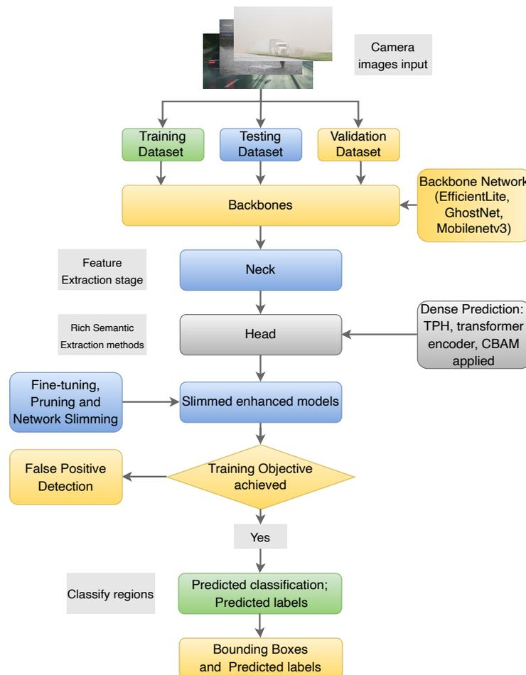
**Figure 4.** Workflow in the proposed one-stage detection model framework.
