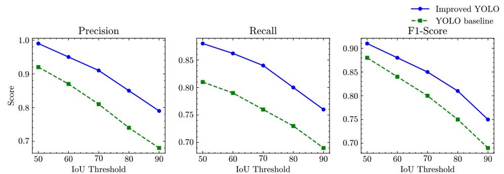
Figure 16. Comparison of improved and baseline models at different IoU threshold (%).
