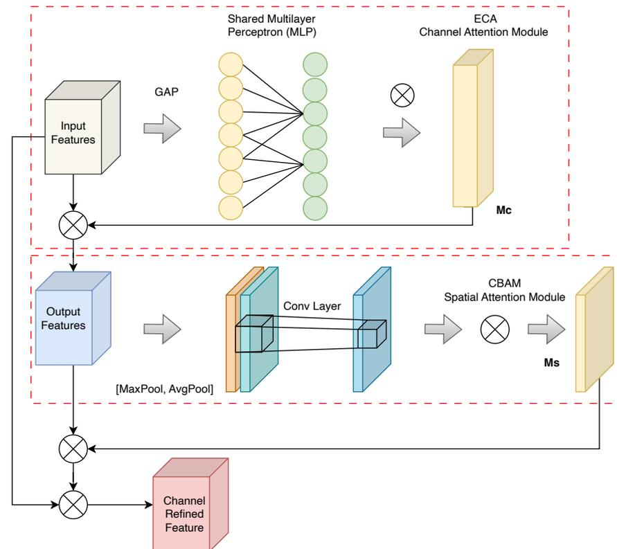
**Figure 9.** The architecture of CBAM in the enhanced YOLOv5 involves the utilization of two consecutive sub-modules, with the additional incorporation of residual paths.
