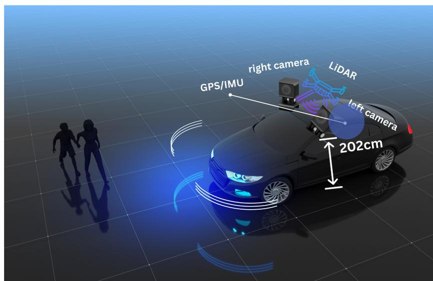
**Figure 1.** The sensor configuration for collecting A2\*D and 3D vehicle platform data on the A\*STAR autonomous driving vehicle includes a spinning Velodyne LiDAR and two color PointGrey Chameleon3 cameras positioned on either side of the LiDAR.
