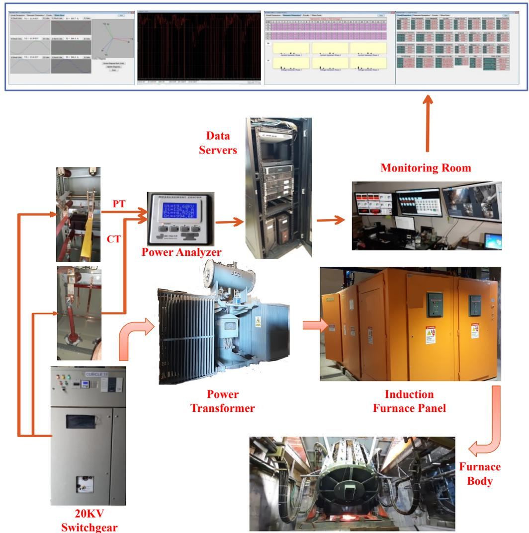
**Figure 3.** The general diagram of the IF system.
