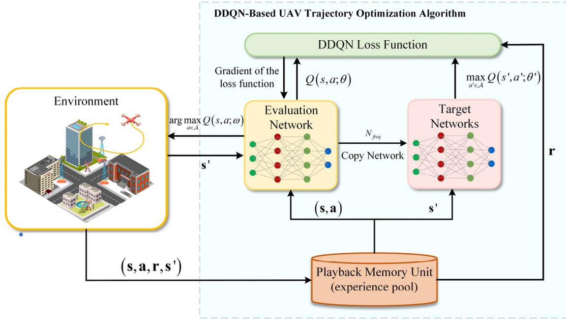
Figure 3. The architecture of DDQN.
