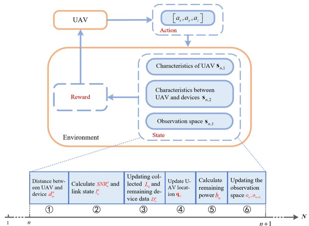
Figure 2. The MDP for trajectory optimization in the data collection scenario.
