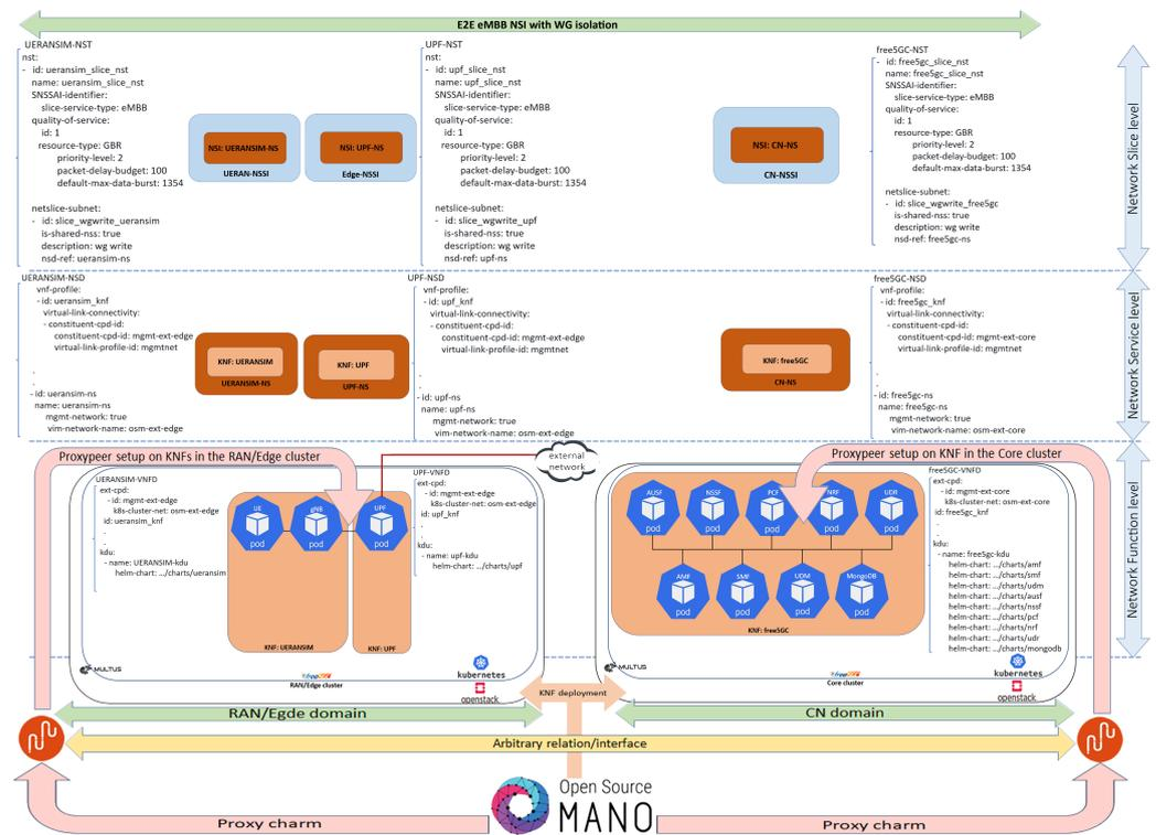
Figure 4. An E2E eMBB NSI with WG isolation created on XVPN-OSM architecture.
