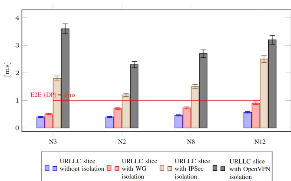
**Figure 5.** Latency comparison at different interfaces in DP and CP while operating an individual URLLC NSI with 2 URLLC UEs per slice.
