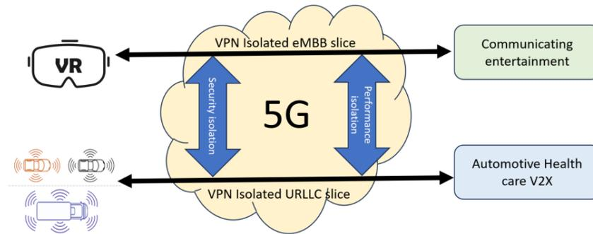
**Figure 1.** VR and automotive V2X applications operate over one eMBB slice and one URLLC slice, respectively, in a slice-isolated 5G network in which performance and security isolation are guaranteed.
