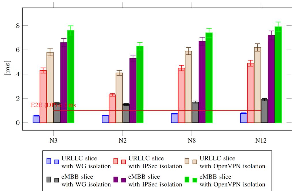
**Figure 6.** Latency comparison of different interfaces in DP and CP while operating two simultaneous URLLC and eMBB NSIs with 2 URLLC UEs and 2 eMBB UEs per slice.
