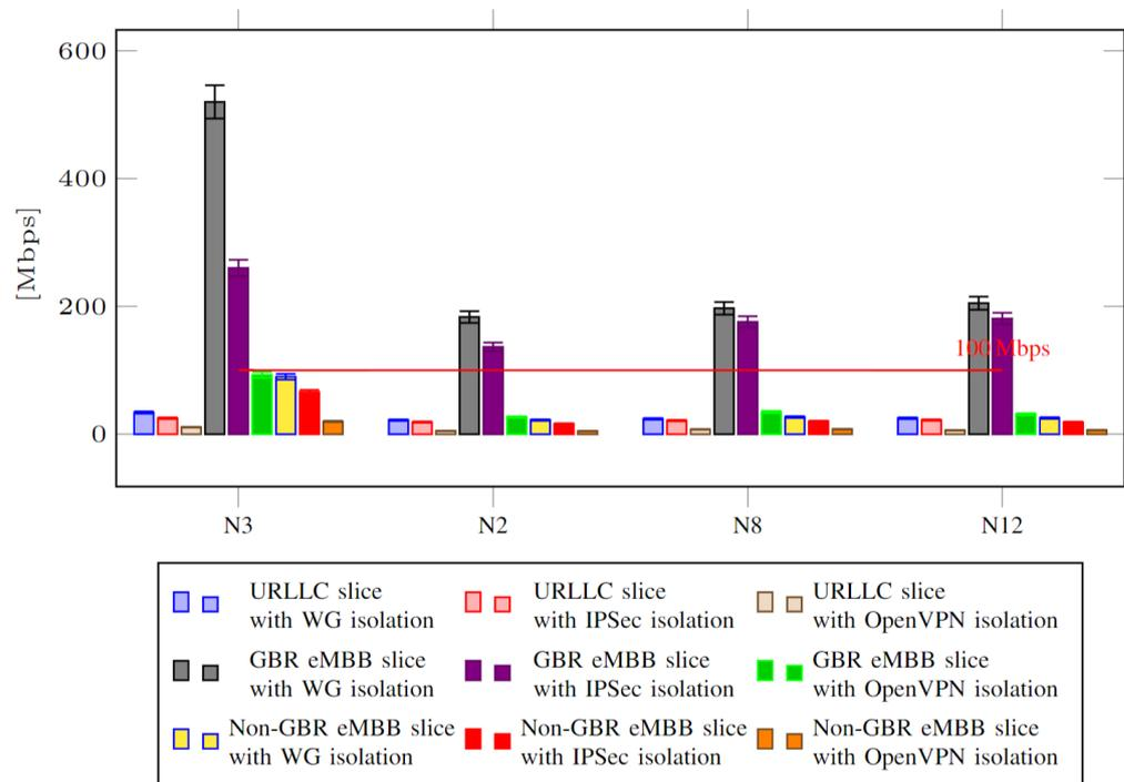
**Figure 8.** Throughput comparison of different interfaces in DP and CP while operating three simultaneous; one URLLC and two eMBB NSIs with 5 UEs per slice.
