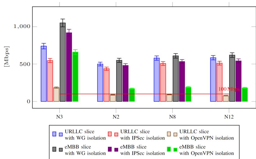
**Figure 7.** Throughput comparison of different interfaces in DP and CP while operating two simultaneous URLLC and eMBB NSIs with two UEs per slice.
