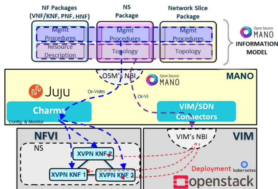
**Figure 3.** The proposed XVPN-OSM framework, where the OSM-NBI and Proxy charms are used to configure different types of NFs deployed on the NFVI [26].
