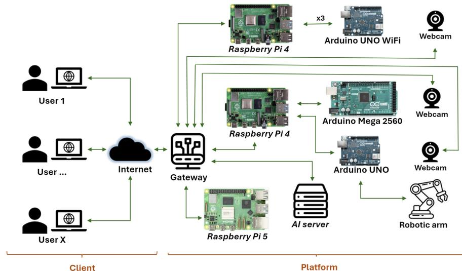
**Figure 2.** Hardware architecture of the Industry 4.0 Remote Platform.
