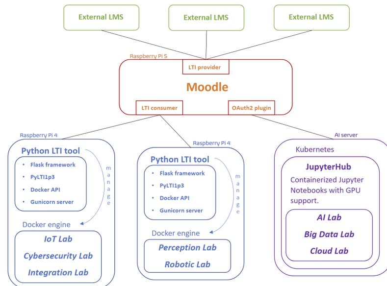
**Figure 1.** Architectural design of the Industry 4.0 Remote Platform.
