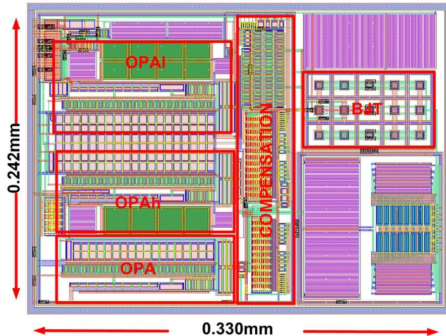
Figure 12. The layout of the proposed BGR with 0.18  $\mu\text{m}$  Bipolar-CMOS-DMOS process.
