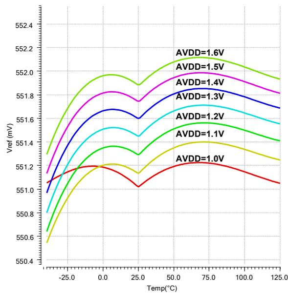
Figure 8. The simulated temperature behavior of  $V_{ref}$  at TT process corner, with varying supply voltage.
