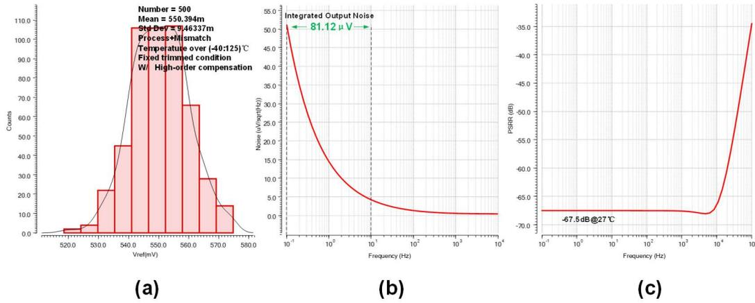
**Figure 10.** (a) The results of the estimated reference voltage output  $V_{ref}$  from 500 Monte Carlo runs under 1 V power supply voltage. (b) The noise spectrum of the simulated bandgap output under 1 V power supply voltage. (c) The simulated PSRR of the BGR circuit under 1 V power supply voltage.
