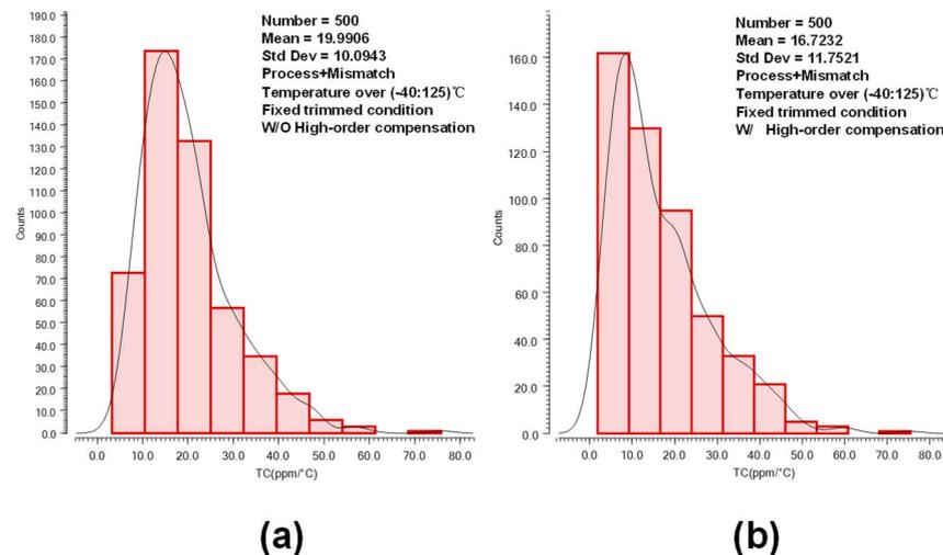
Figure 9. (a) The estimated TC results without high-order compensation from 500 Monte Carlo runs under 1 V power supply voltage. (b) The estimated TC results with high-order compensation from 500 Monte Carlo runs under 1 V power supply voltage.
