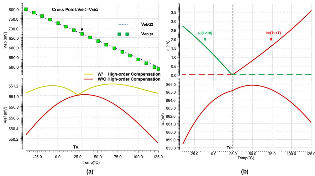
**Figure 3.** (a) The curve of  $V_{ebQ3}$ ,  $V_{ebQ2}$  and  $V_{ref\_1st}$  with varying temperatures. (b) The curve of load current,  $I_{Q3}$ , of Q3 and the compensation,  $I_c$ , with varying temperatures.
