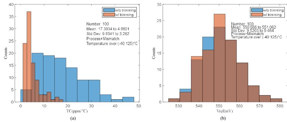
Figure 11. (a) The estimated TC results w/trimming compared with TC results w/o trimming from 100 Monte Carlo runs under 1 V power supply voltage. (b) The estimated  $V_{ref}$  results w/trimming compared with TC results w/o trimming from 100 Monte Carlo runs under 1 V power supply voltage.
