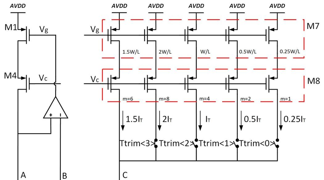
Figure 7. Trimming network of  $(W/L)_{M7}$ .
