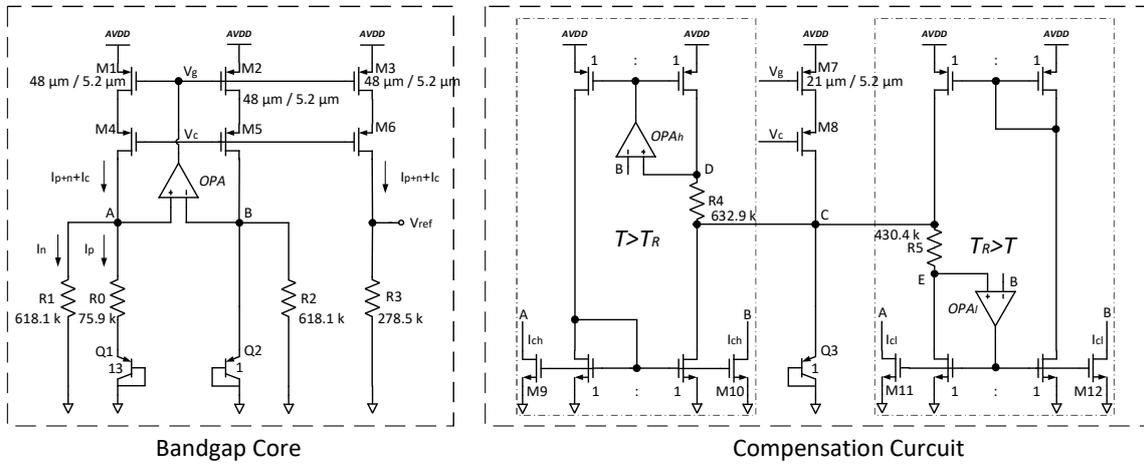
Figure 2. Schematic of proposed low-voltage BGR with high-order compensation.
