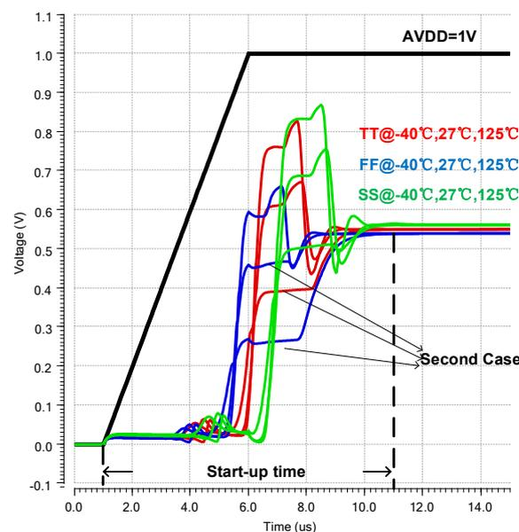
Figure 6. Simulated start-up waveforms of the proposed BGR.
