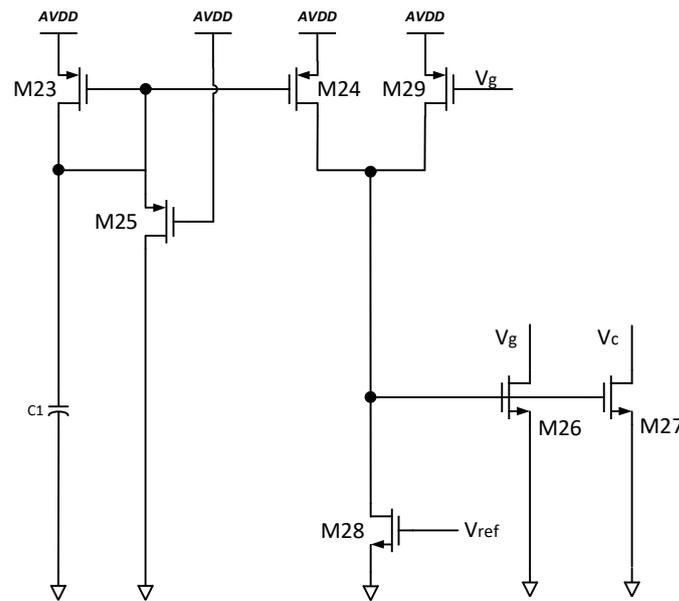
Figure 5. Start-up circuit.
