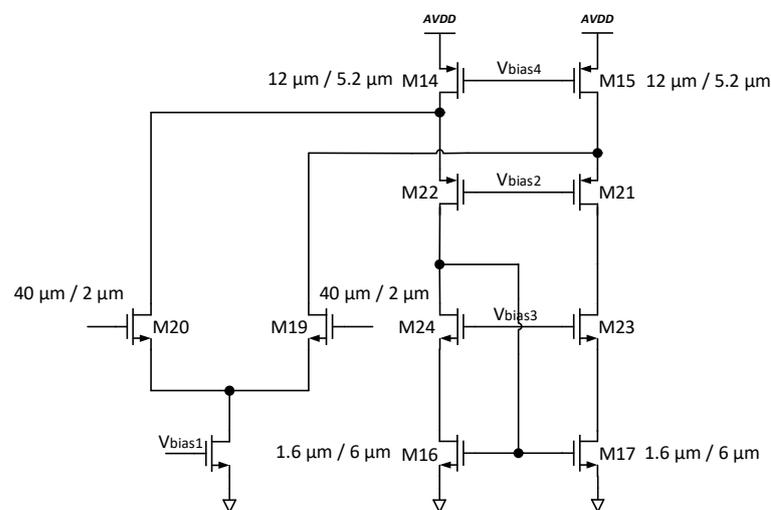
Figure 4. Schematic of the OPA used.
