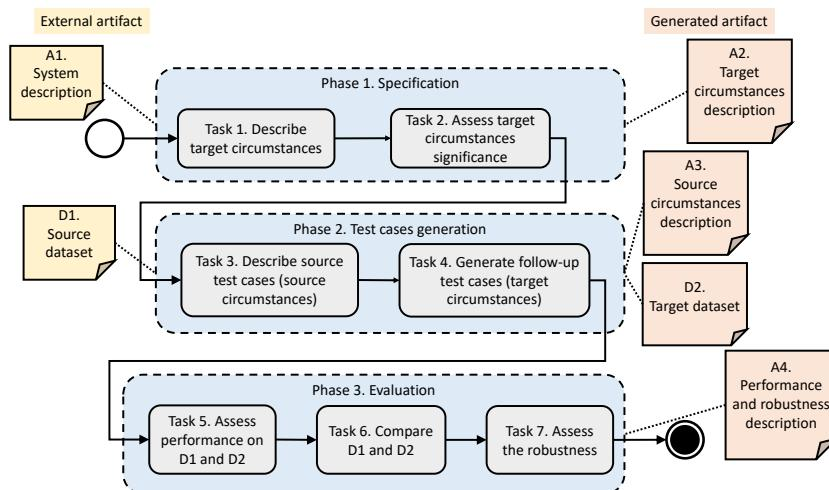
**Figure 5.** Business Process Model and Notation (BPMN) diagram of the robustness testing method. Yellow artifacts (A1 and D1) are external data, provided by the developer of the system, while orange artifacts are generated during the tasks.
