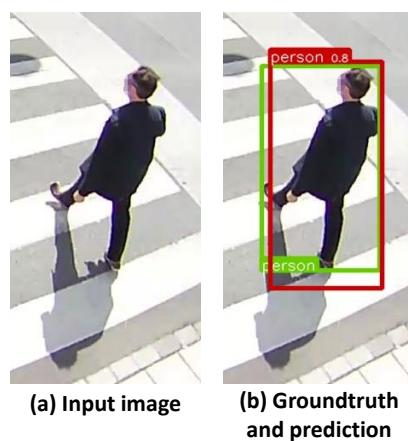
**Figure 1.** Detection of an object (person) on a pedestrian crossing. In green, the groundtruth (true location and true class); in red, the predicted bounding box and class (with confidence score).
