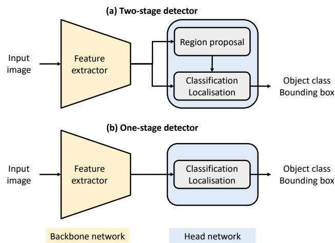
**Figure 2.** Overview of (a) a two-stage detector and (b) a one-stage detector.
