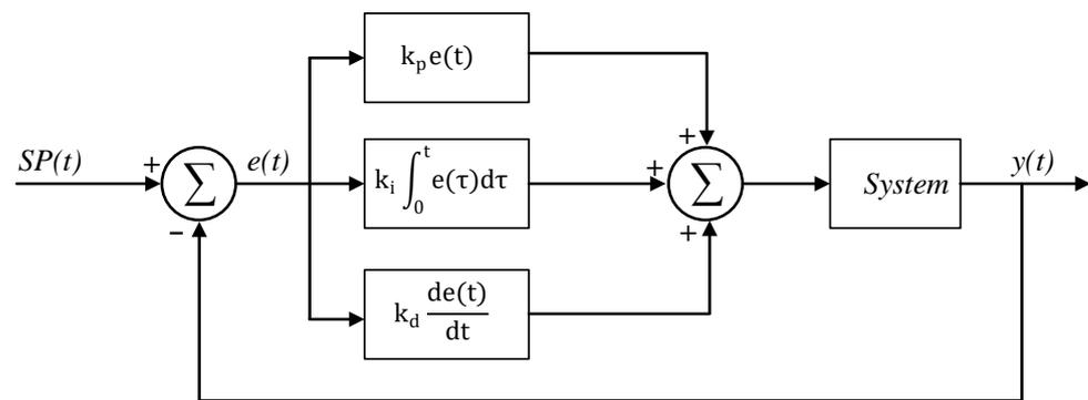
**Figure 3.** Scheme of a PID controller to track the system output to a desired point.
