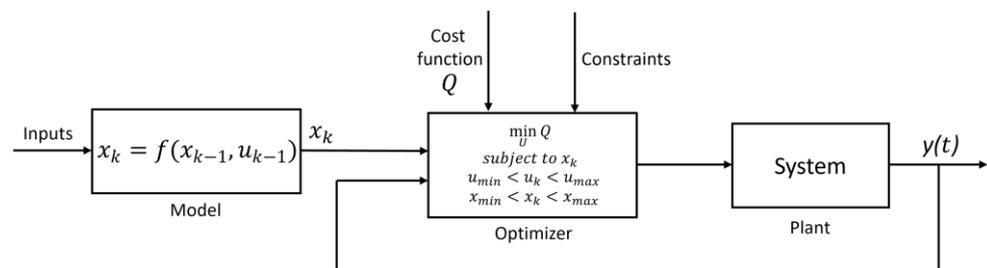
**Figure 5.** Diagram of the interconnections among the model, optimizer, and system of an MPC controller technique.
