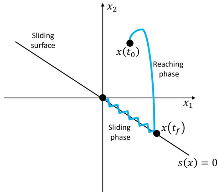
**Figure 4.** Schematic of the sliding surface of an SMC strategy.
