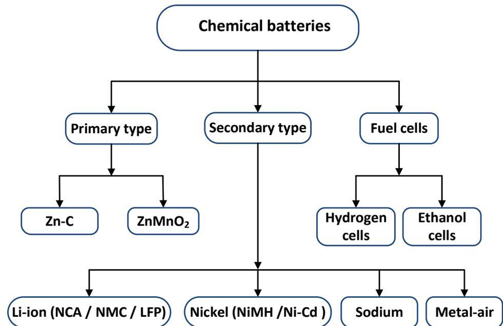
**Figure 1.** Classification of electrochemical batteries.
