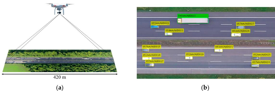
**Figure 7.** The schematic diagram for the HighD dataset. (a) The length of the section is about 420 m; (b) information of the vehicles in the HighD dataset.
