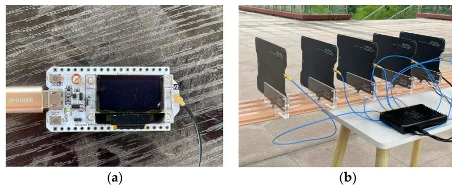
**Figure 1.** Hardware diagram of the LoRa data acquisition module: (a) LoRa transmitting node, and (b) receiving antenna array.
