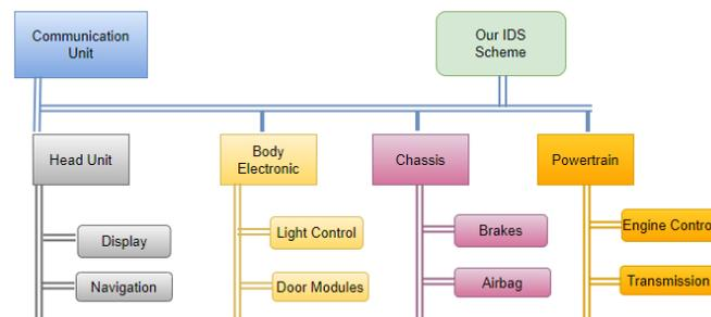
**Figure 3.** The architecture of the in-vehicle network with our proposed scheme integrated.
