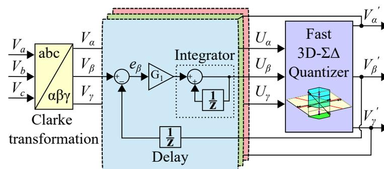
Figure 2. Three-dimensional sigma-delta modulation loop. The nominal value of all gains is unity.
