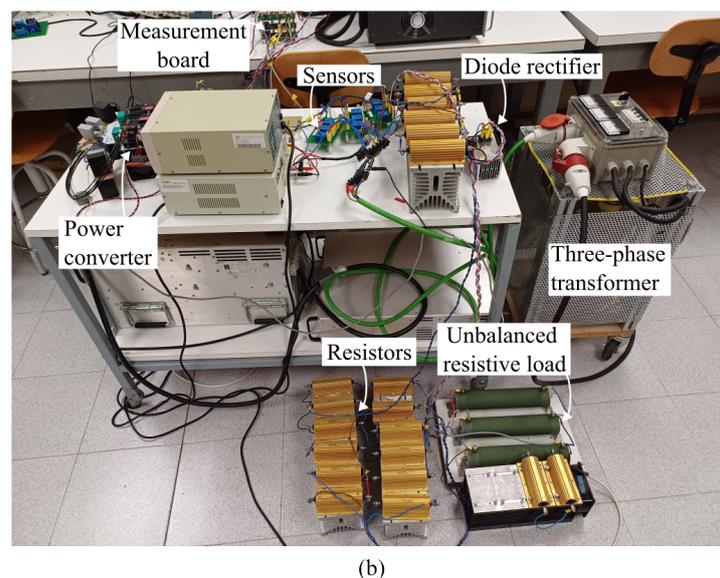
Figure 9. View of the experimental setup: (a) schematic; (b) photographic depiction.
