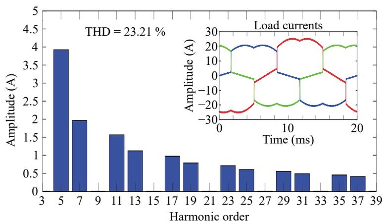
**Figure 6.** Characteristics of the simulated load.
