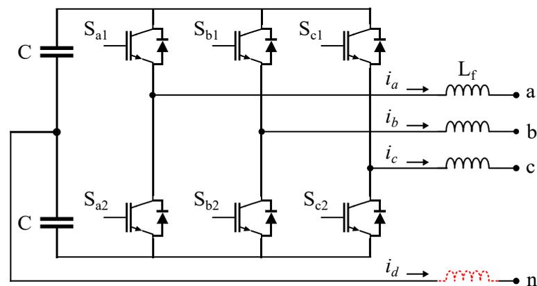
**Figure 1.** Three-leg four-wire voltage source converter. The red dashed line indicates the option for connecting an optional inductance to the neutral wire.
