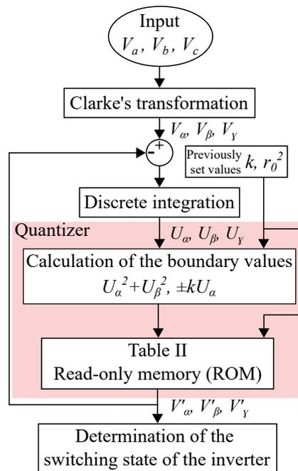
**Figure 4.** Flowchart of the proposed 3D- $\Sigma\Delta$  technique.
