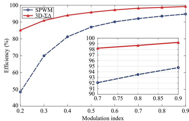
**Figure 8.** Experimental converter efficiency curves at  $f_{max} = 200$  kHz.
