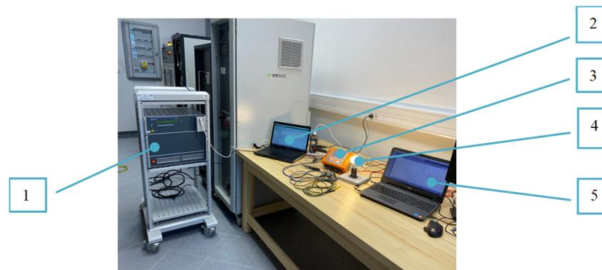
**Figure 13.** Test stand for testing LED lamps: 1—programmable voltage source; 2—PC with installed specialised software to control the power source; 3—power quality analyser; 4—luminaire with the LED lamp under test; 5—PC with installed specialised software working with the power quality analyser.
