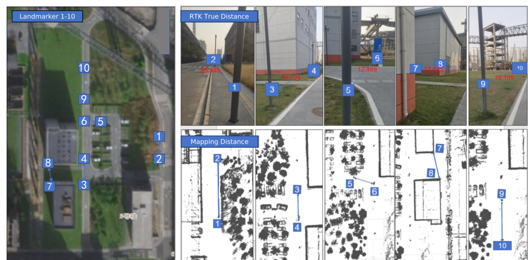
Figure 2. The experimental environment in an industrial park and five sets of landmarks used to evaluate the accuracy of mapping.
