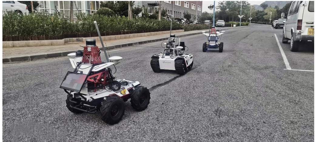
Figure 1. The three mobile robots equipped with RoboSense Lidar-16, NOVATEL OEM7 RTK, and IMU in an industrial park.
