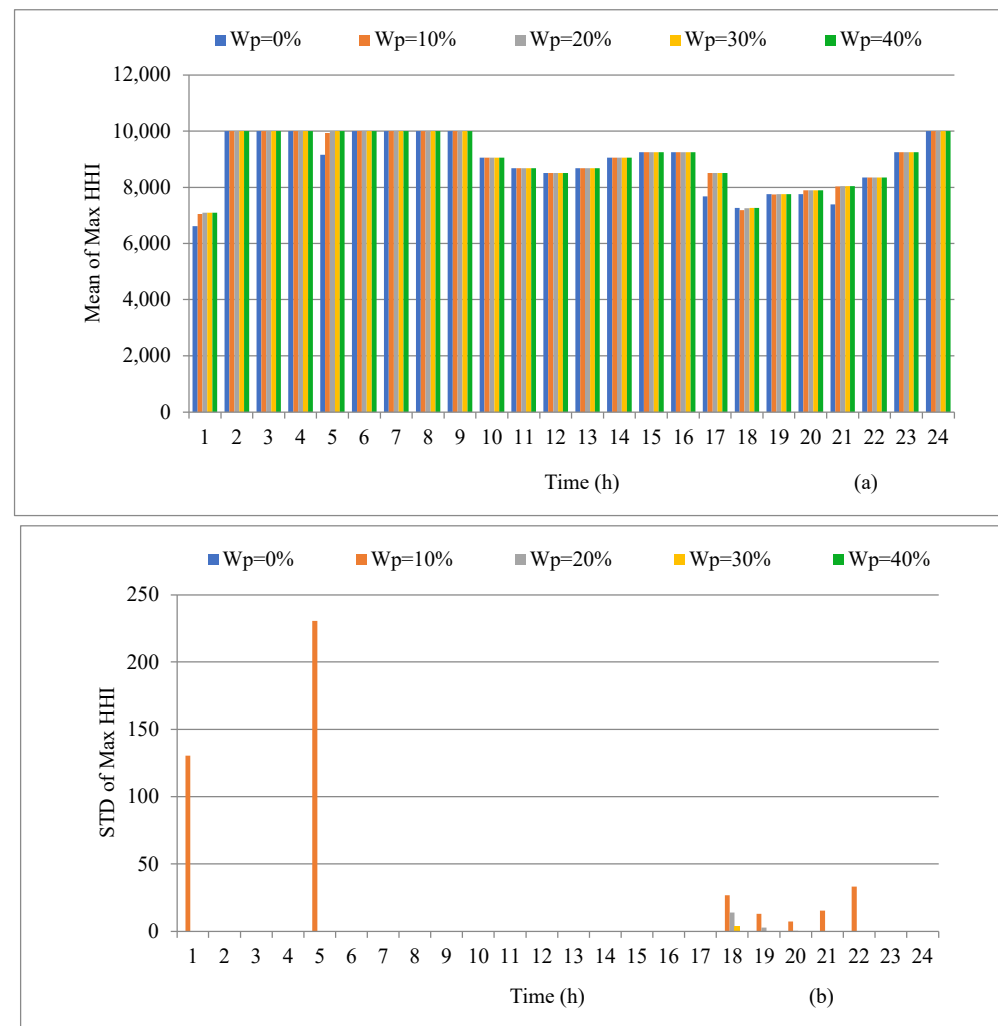
Figure 16. Maximum value of HHI with increasing level of wind penetration in average load level for (a) mean, (b) STD.
