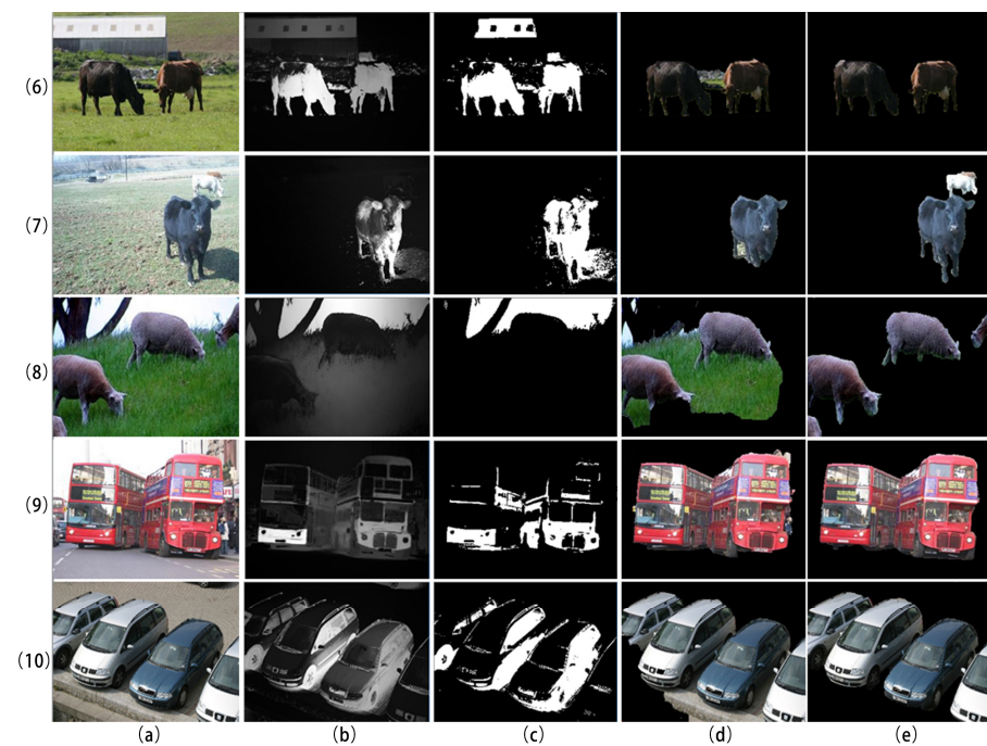
Figure 6. Comparison of multi-target segmentation results. (a) Original input image, (b) salient object detection result, (c) binary image obtained after using min_cut segmentation on the salient image, (d) result of 20 iterations of GrabCut algorithm segmentation, and (e) segmentation result of the improved GrabCut algorithm.
