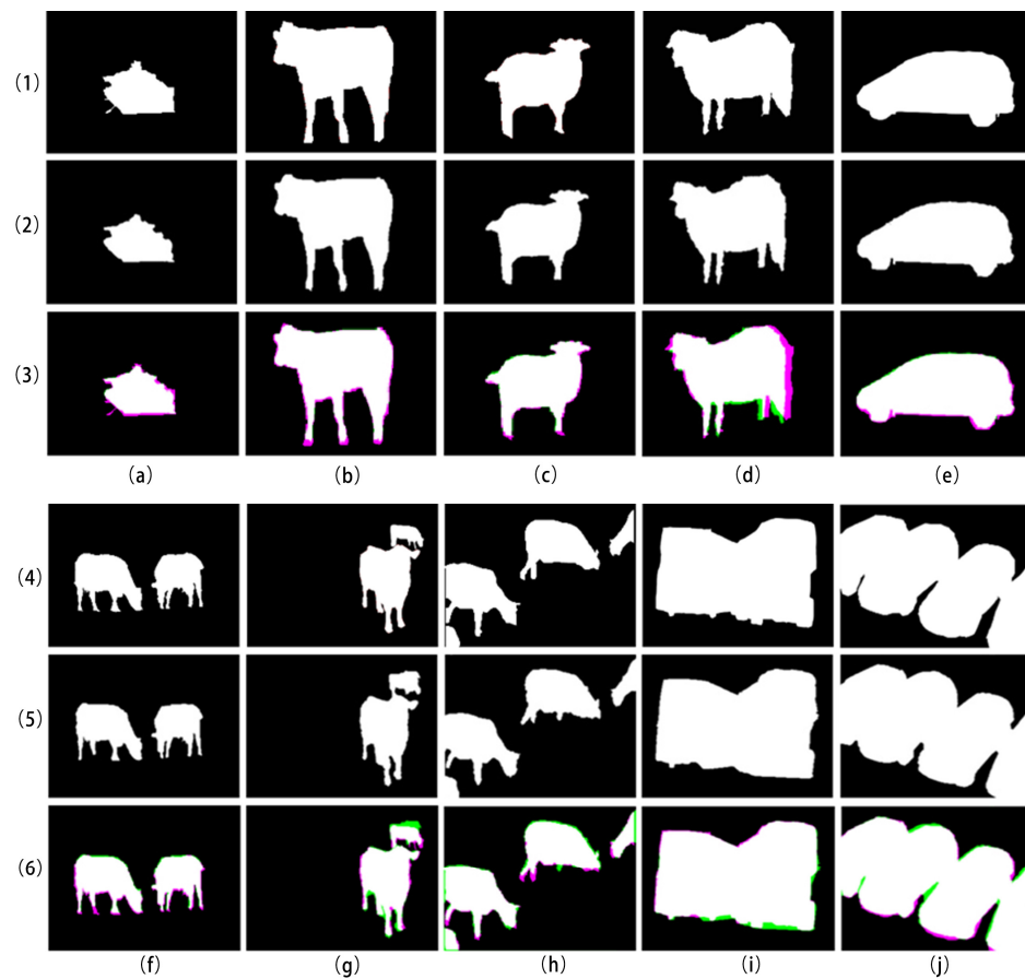
Figure 7. The residual error between the automatic segmentation result and the target image. (1) The true value image of a single target original image, (2) the true value image automatically segmented from a single target image, (3) the residual image of single target image segmentation, (4) the true value image of a multi-target original image, (5) the true value image automatically segmented from a multi-target image, and (6) the residual image of multi-target image segmentation.
