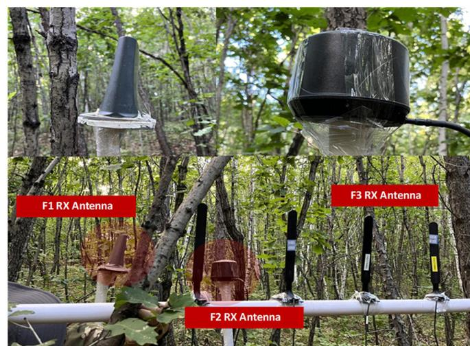
Figure 4. Deployment of measurement receiving-end antenna in Dongshan dense coniferous forest.
