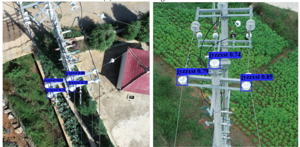
(c) Insulator tie wire loosening test results
