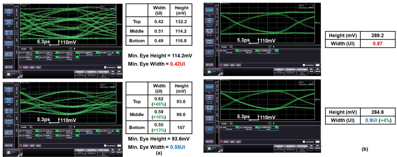
Figure 8. Measurement result of eye diagram when the eye enhancement is (top) off and (bottom) on: (a) at 56 Gb/s PAM-4; and (b) 28 Gb/s NRZ.
