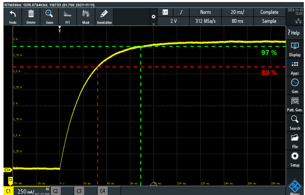
Figure 19. Obtained experimental results when the reference current changes from 1 to 3 A.
