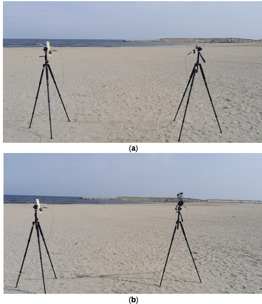
Figure 12. Antenna setup for on-drone gain measurements in an OATS: (a) horizontal, off-drone face-to-face antennas as a reference; (b) horizontal, on-drone face-to-face antennas.
