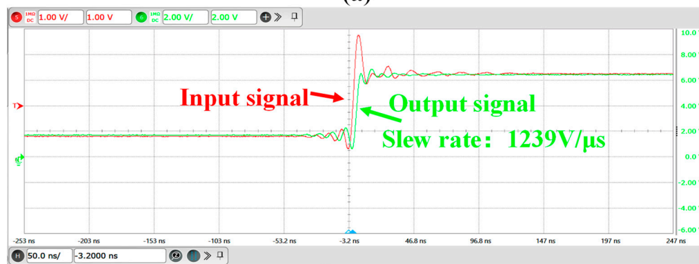
Figure 16. Measured step responses of the proposed LA with the SRE circuit: (a) fall condition and (b) rise condition.
