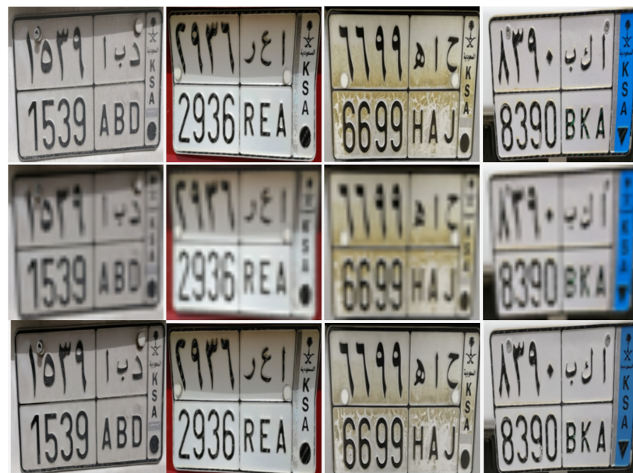
Figure 6. Comparison of image resolutions: (top row) original HR image ( 192 \times 192 ), (middle row) downsampled LR image ( 48 \times 48 ), and (bottom row) super-resolved image ( 192 \times 192 ) generated using the Diffusion Model.
