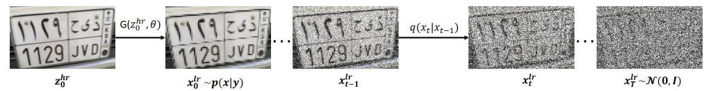
Figure 2. The forward process for adding noise until a completely noisy image is obtained.
